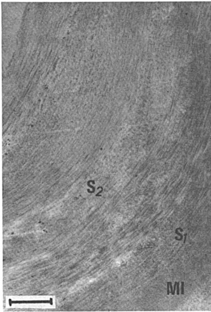
Figure 13. Avicelase 1 + mannanase treatment. Degradation of S 2 in an earlywood tracheid showing lamellar aggregation pattern. Scale = 1 μm.
