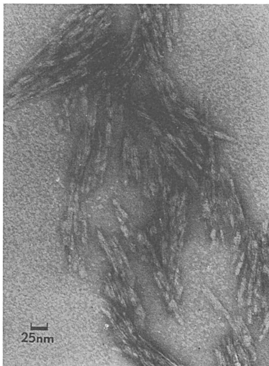
Figure 4. Electron micrograph of cellulose from beechwood, boiled with 2N TFA for 2 hr and subsequently with 5N TFA for 5 hr. Negative staining with uranyl acetate.
