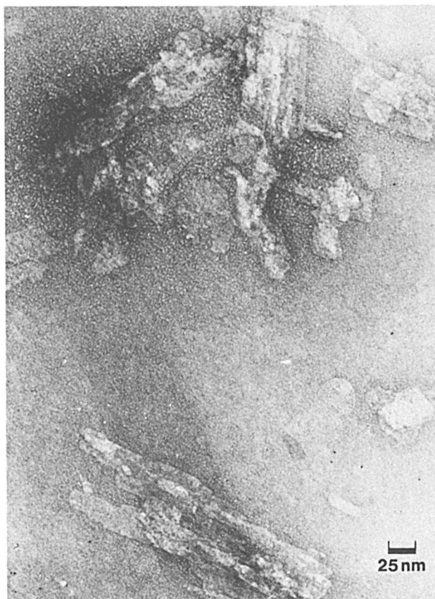
Figure 5. Electron micrograph of cellulose from beechwood, dissolved in 100% TFA at 120°C, precipitated, and boiled with 2N TFA for 6 hr. Negative staining with uranyl acetate.
